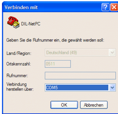
Figure 5: Direct Connection Set-up with HyperTerminal
