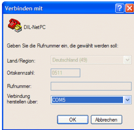
Figure 5: Direct Connection Set-up with HyperTerminal
