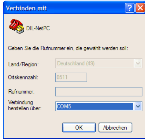
Figure 6: Direct connection setup with HyperTerminal
