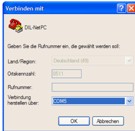
Figure 6: Direct connection setup with HyperTerminal
