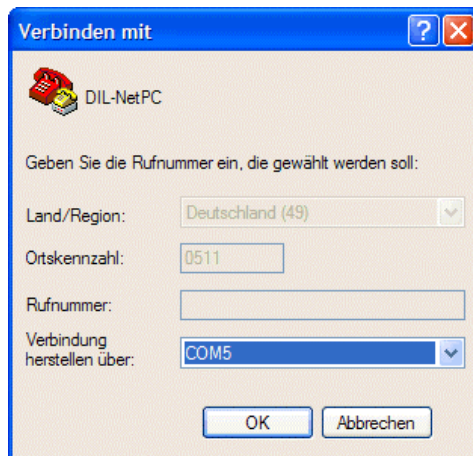
Figure 5: Direct Connection Set-up with HyperTerminal
