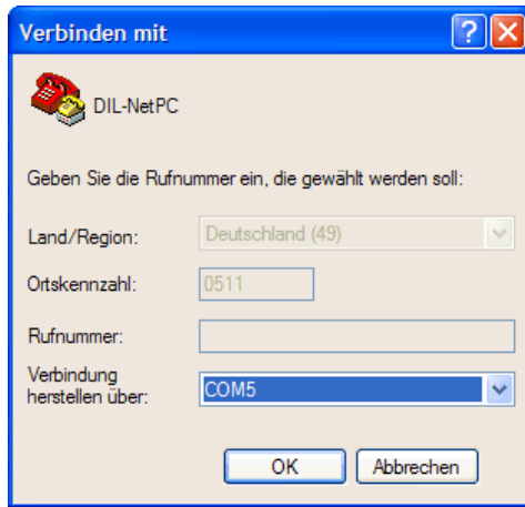
Figure 5: Direct Connection Set-up with HyperTerminal
