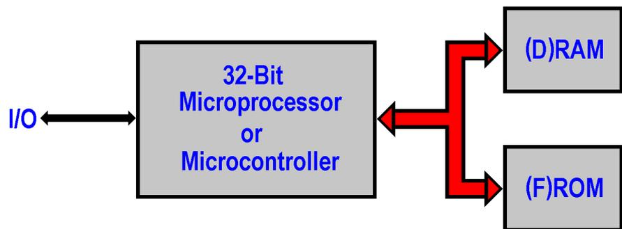
**Figure 2:** Block Diagram for a minimum Linux Hardware
