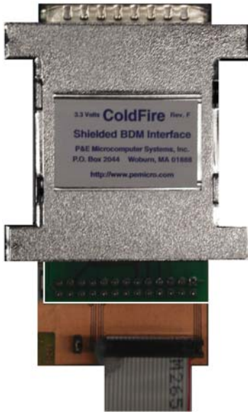
Picture 3: Connection between P&E BDM Interface and SSV BDM Interface Adapter
